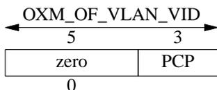
May only be used when **vlan\_vid** is not wildcarded and does not exact match on 0 (which only matches when there is no 802.1Q header).
