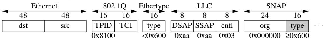
When a packet doesn't match any of the header formats described above, Open vSwitch and OpenFlow set this field to **0x5ff** (**OFP\_DL\_TYPE\_NOT\_ETH\_TYPE**).
